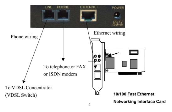
The RJ-11 port supports 10 Mbps connections. When inserting a RJ-11 plug, be sure the tab on the plug clicks into position to ensure that it is properly seated.
