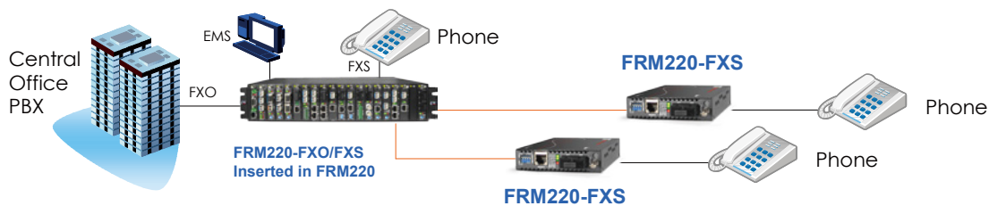
Figure 3 : Selectable FXO or FXS mode
