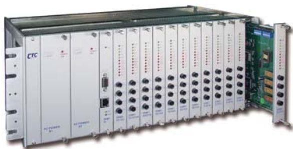
4U, 19", 13-slot E1 and Fractional E1 Concentrator With SNMP Management
