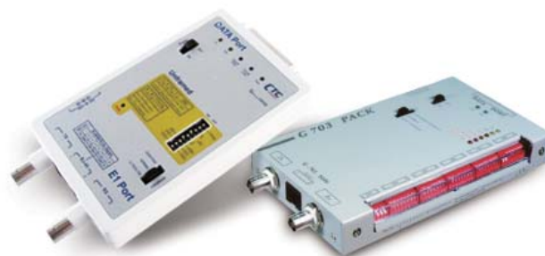
Compact-size, Single-port E1/Fractional E1 Access Unit
