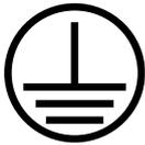
2. When supplying power to this equipment, connect the accessory 3-pin power cord to a 3-pin grounded power outlet. If a grounded 3-pin outlet is not available, before supplying power to the equipment, use a conversion adapter and ground the green wire, or connect the frame ground on the rear panel of the equipment to ground. If power is supplied without grounding the equipment, there is a risk of receiving a severe or fatal electric shock.
