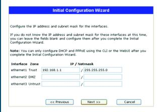
To change the IP address of the Trust zone interface, enter a new IP address and netmask. If you change the IP address and netmask of the Trust zone interface, then your workstation and the Trust zone interface of the NetScreen-50 might be in different subnetworks. To manage the NetScreen-50 with the WebUI, ensure that your workstation and the NetScreen-50 are in the same subnetwork. Click **Next**.
